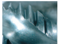
■ Cutting edge after 1.000 holes Tapping
